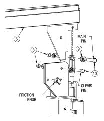
Remove the friction knob from top of the mast. Place the swivel sailfin plate on the rear boom arm between the two mounting plates on the top of the mast assembly. Install the main pin first. Place 2 plain washers under the head of the bolt and 2 under the lock nut. Tighten the lock nut completely and then back the lock nut off 1 full turn for the main pin, back the lock nut 2 full turns off for the clevis pin. Reinstall the friction control knob.
