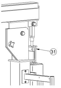
Loosen the friction control knob until the desired boom balance is obtained. Again if the boom does not balance as desired, follow the provided boom balancing instructions. But only after reinstalling the spring rod shipping support.
