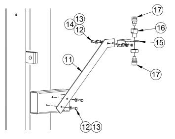
Install the conduit bracket to the mast using two 1/4"-20 x 1.00" bolts and washers provided. After the bracket is in place, completely tighten the bolts. Install the bulkhead bracket, bulkhead adapter and quick disconnect to the conduit bracket. Repeat this step for the opposite side if necessary.
