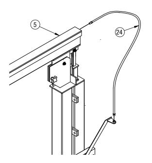
Mount conduit through cable trough. Connect the conduit to quick disconnect on the feeder and the other end to the quick disconnect on the bukhead bracket. Repeat this step for the opposite side if necessary.
