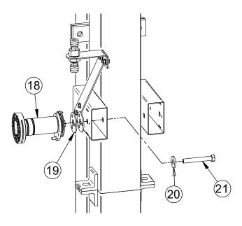
Remove original .625" bolt from the Spindle Assembly. Place two additional friction washers under the spindle. Install the spindle assembly using the 1/2"-13 x 3.00" bolt and washer provided. Line up the small hole on the spindle assembly with the roll pin on the mast. After the spindle assembly is in place, completely tighten the bolt. Repeat this step for the opposite side if necessary.
