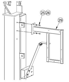
Install the control box mounting bracket to the mast using two 1/4"-20 x .75" bolts and washers provided. This bracket may be mounted on either side of the mast.
