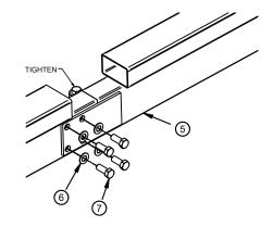
Support the hinge end of the boom on a box or stool such that the boom arm is parallel to the floor. Remove protective wrap on the hoses and cables at the hinge joint. Rotate the back end of the boom on the hinge to close the flange against the boom arm. Insure that the cables and hoses at the joint do not get pinched or damaged. Install the four 1/2-13 bolts and washers, and torque to 48-52 ft-lb. Torque the hinge bolt to 48-52 ft-lb.
