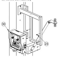
Partially thread the four #10-24 thread forming screws into the mounting bracket, allowing 1/16" between the head of the screw and the bracket. Insert the keyholes on the back of the control box over the screw heads and slide the box downward to secure it. Connect the control box to the control cable that leads out of the boom.
