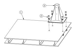
Mount the pedestal to the pallet base using four  $3/4-10 \times 2^{\circ}$  bolts, nuts and washers (not provided). If a pallet base is not used, mount the pedestal directly to a solid concrete floor. Use four  $3/4^{\circ}$  concrete anchors (not provided) with washers.
