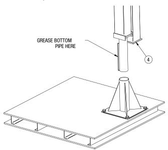
• Coat the bottom pipe with grease. Insert the mast assembly into base.
