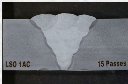
单丝LSO埋弧焊 AC (板厚:40mm)
