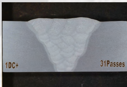
单丝埋弧焊 DC+ (板厚:40mm)
