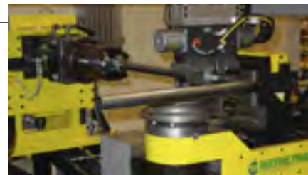
Seatback manufacturing system utilizing 1500RD CNC bend heads
