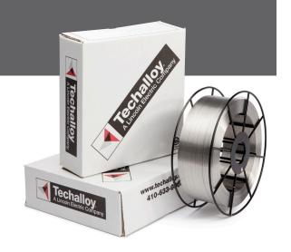
**Techalloy**® **347** electrodes are niobium stabilized stainless steel electrodes used for the welding of types 347 and 321 stainless and stainless clad steels. The addition of niobium reduces intergranular corrosion in severe operating conditions.
