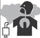
1.b. Operate engines in open, well-ventilated areas or vent the engine exhaust fumes outdoors.
