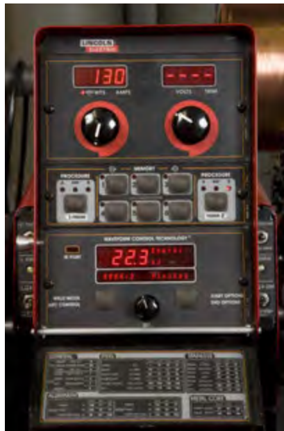
True Energy™ results can be displayed on a Power Feed™ series wire feeder.
