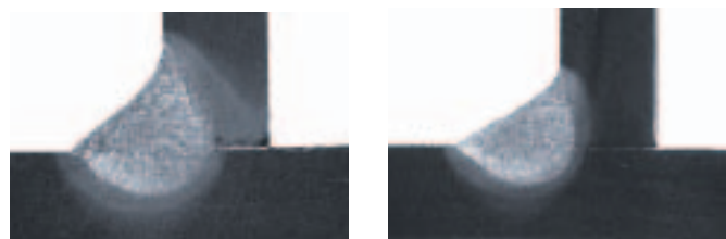
Figure 14 The weld on the left is with DC+. The weld on the right is with AC 25% Balanced, (-)10% Offset, 60Hz.
