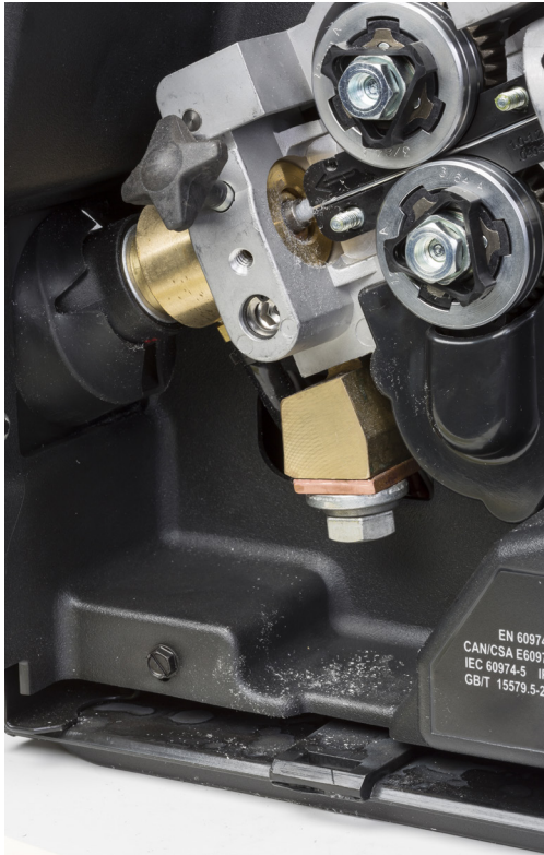
Wire shavings during the feeding process with standard aluminum wire versus SuperGlaze HD
