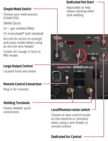
Less arc control (less pinch) in short arc wire processes to decrease spatter
