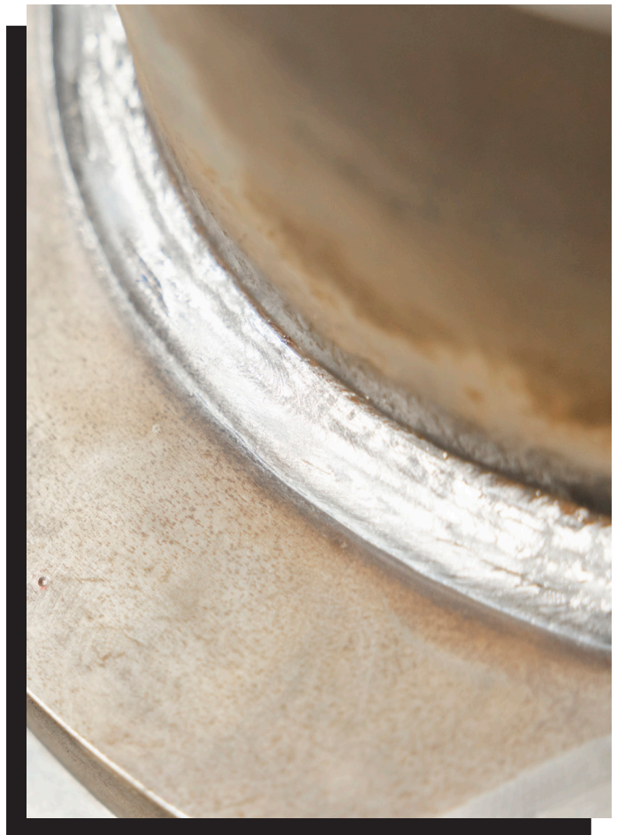
A final HyperFill welded part
