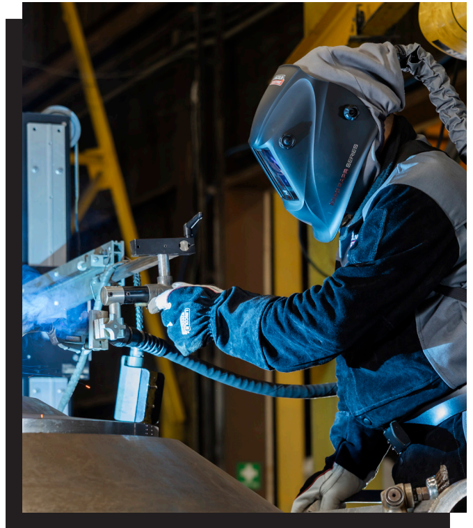
Arroyo welding with HyperFill
