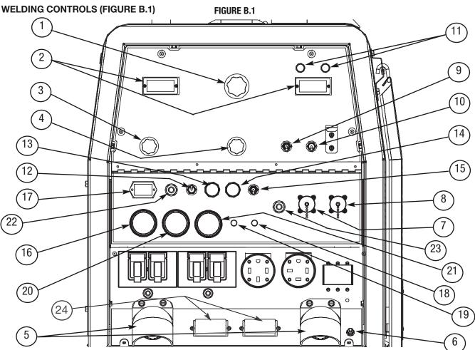
**1. OUTPUT CONTROL**- The OUTPUT dial is used to preset the output voltage or current as displayed on the digital meters for the five welding modes. When in the Arc Gouging or CV-WIRE modes and when a remote control is connected to the 6-Pin or 14-Pin Connector, the auto-sensing circuit automatically switches the OUTPUT CONTROL from control at the welder to the remote control.
