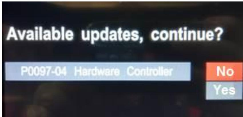
8. After uploading the device will reset itself and this is the end of update. You can also check the upgraded software version in the **System Info** menu – highlight the **Wire Drive** description, the **P0097-04** number (or higher) should appear.
