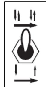
Place the toggle switch in the DOWN position for 2 Step operation or in the UP position for Trigger Interlock operation.
