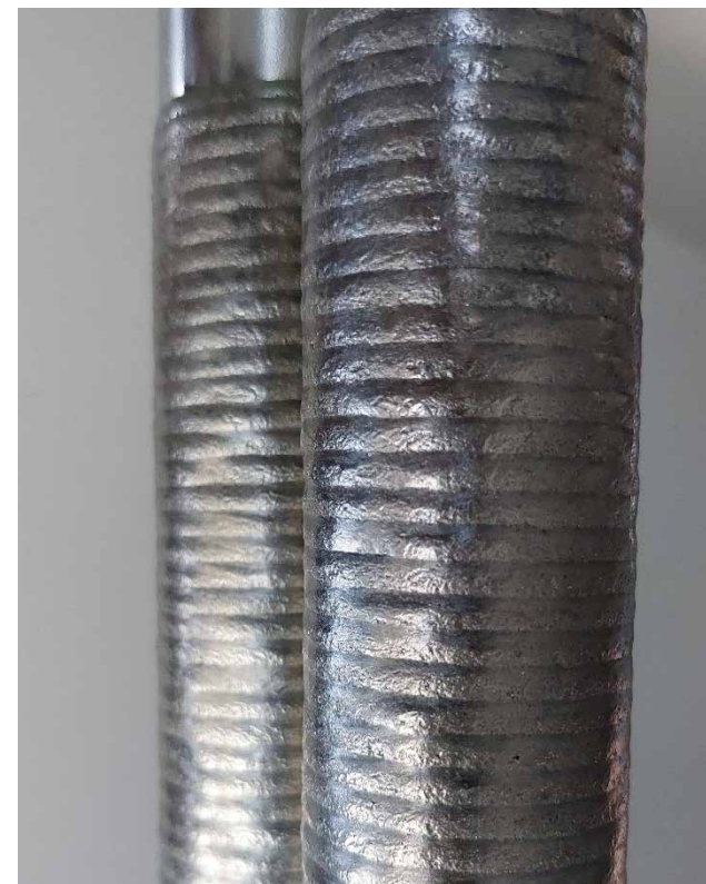
Cladding sample with Precision Power Laser™ 7.5kg/h deposition rate with 4000W of laser power
