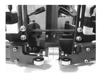
The troggle clamp allows to maintain the carriage against the profil to be welded.
