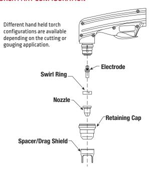
**NOTE:** It is normal for the electrode and nozzle to wear during operation. It is recommended that the Electrode and Nozzle be replaced as a complete set.
