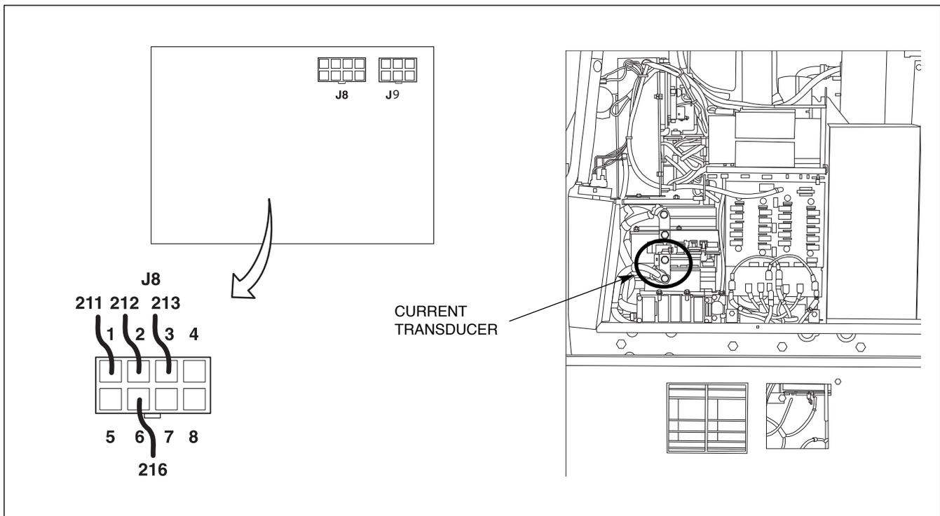
5. Check the DC supply to the Current Transducer at the following points:
