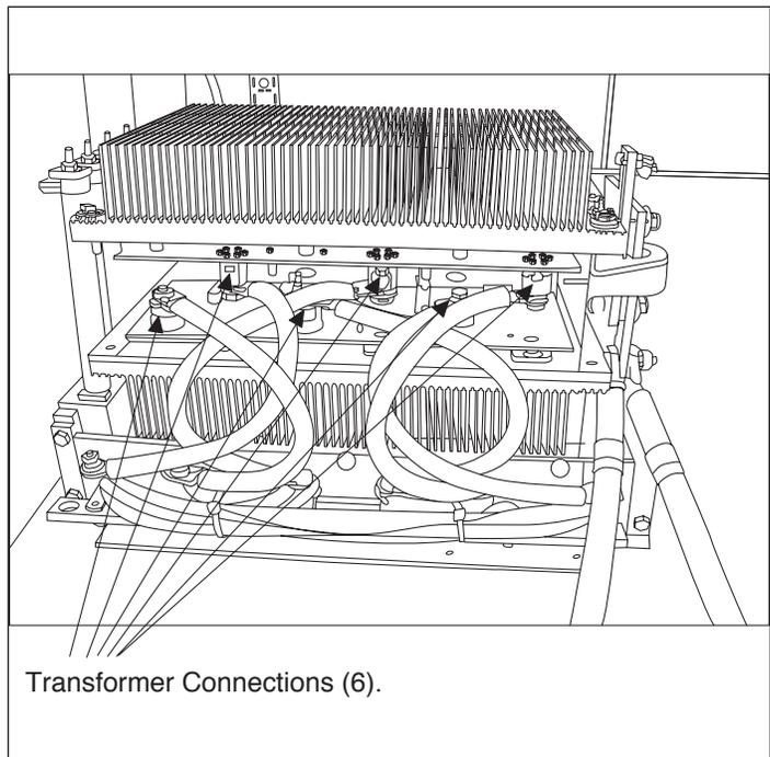
**FIGURE F.13 – RECTIFIER RESISTANCE CHECK**
