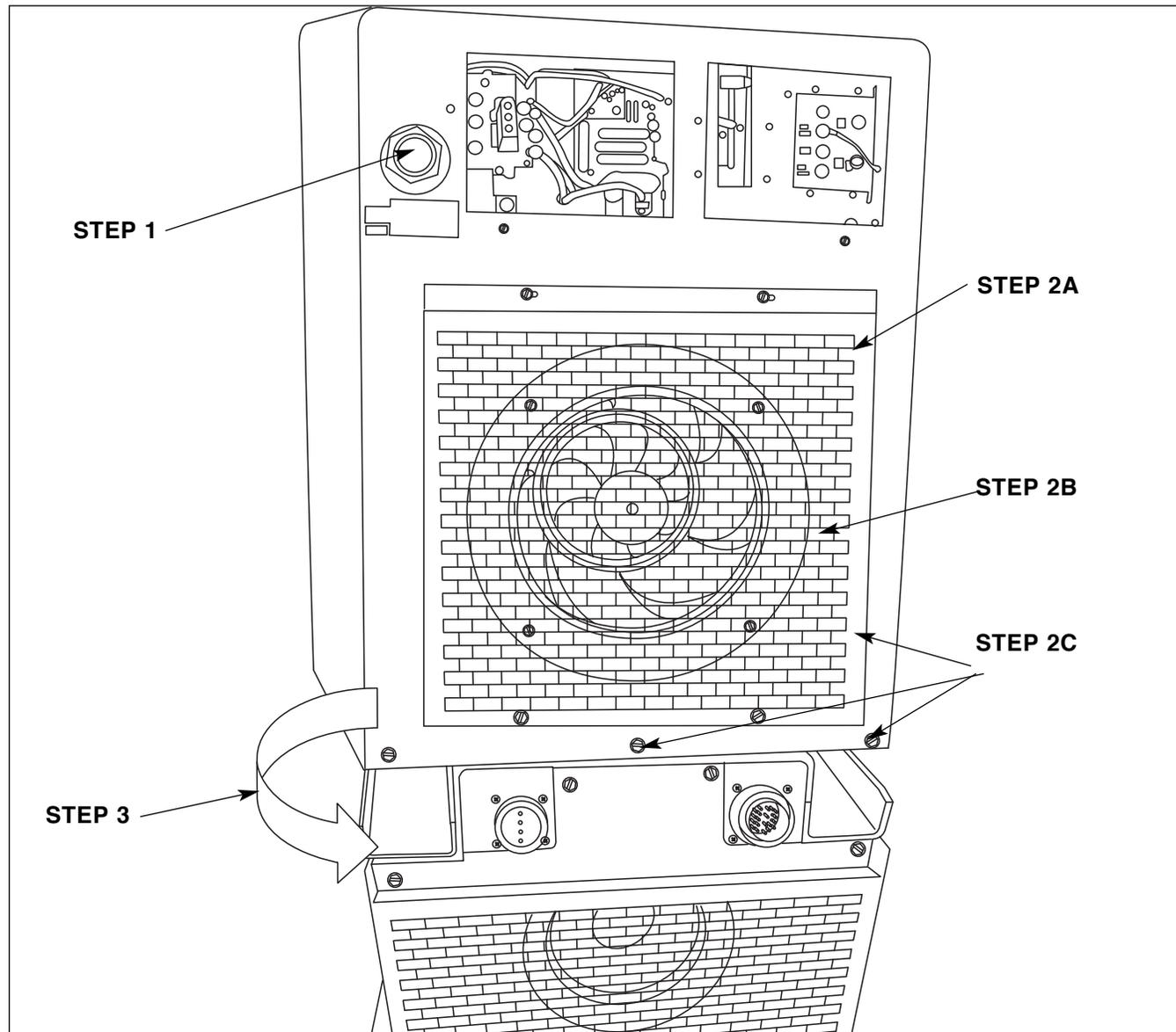
**STEP 1:** After disconnecting the input power, disconnect the input leads from the 1CR contactor.
