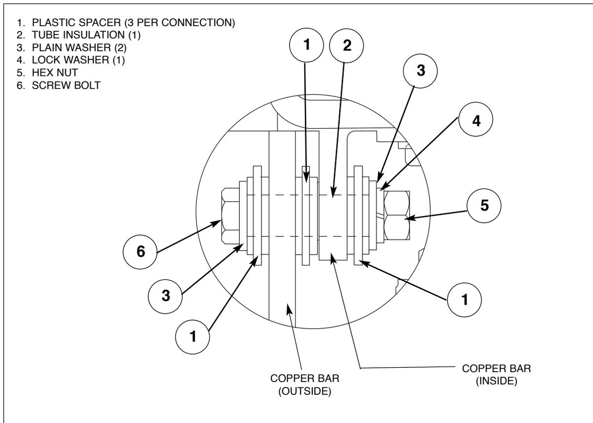
Assemble in reverse order with the “transducer indicator arrow” pointing down when in the installed position. After installing the copper bars back through the transducer, ensure that the copper bars are insulated from each other BEFORE reconnecting them to the Output Rectifier.
