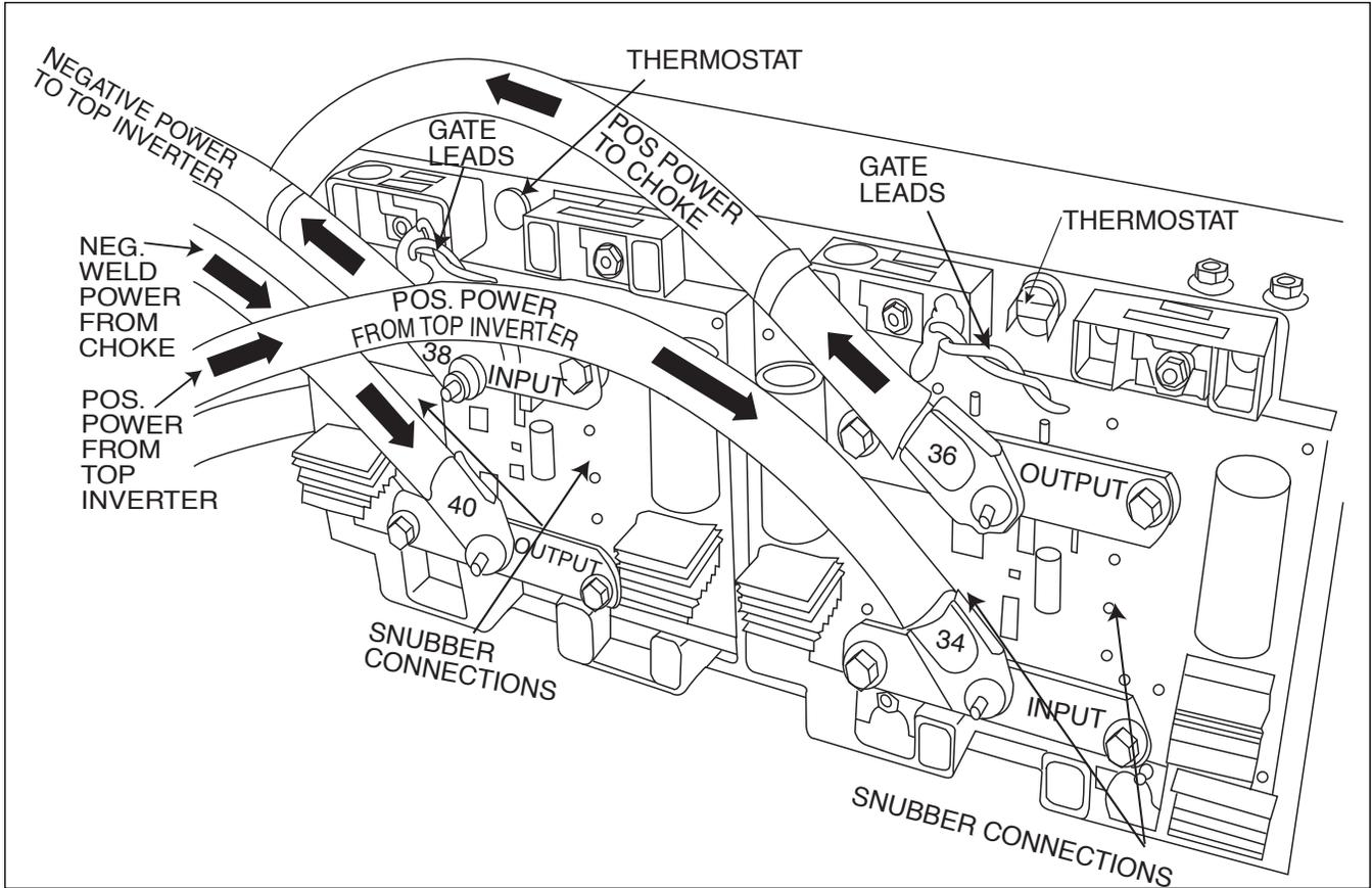
One of two AC Switch Chopper Assemblies (left side shown)
