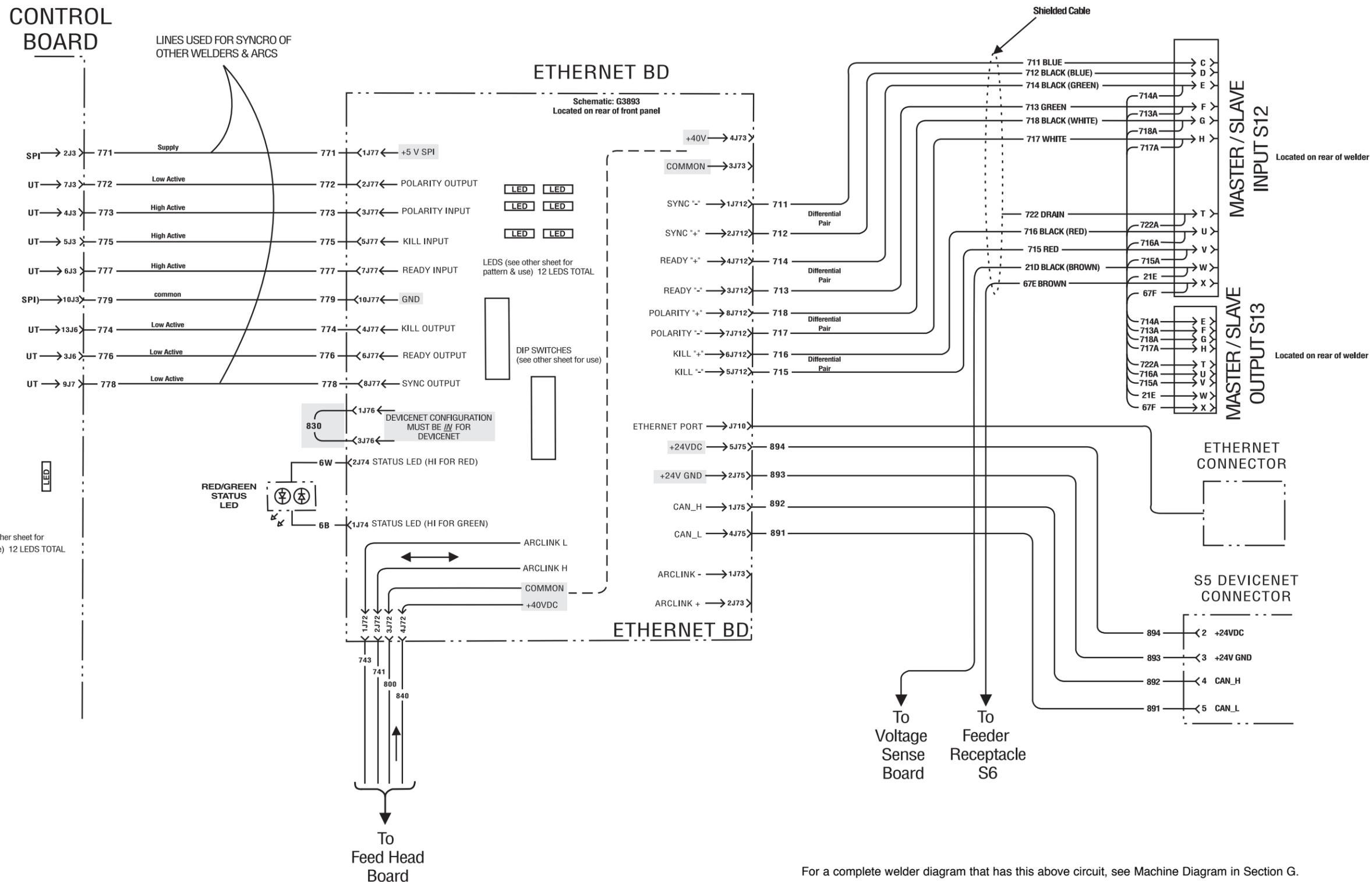
For a complete welder diagram that has this above circuit, see Machine Diagram in Section G.
