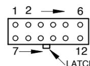
VIEW OF CONNECTOR ON PC BOARD
