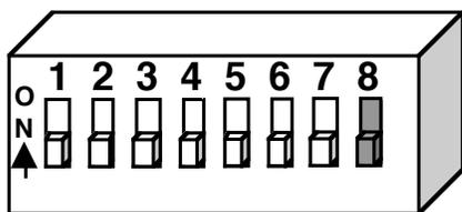
5. Replace the cover and screws. The PC board will "read" the switch at power up, automatically adjusting all control parameters for the speed range selected.
