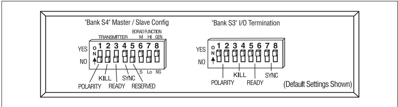
FIGURE F.47 – ETHERNET PC BOARD SET-UP
