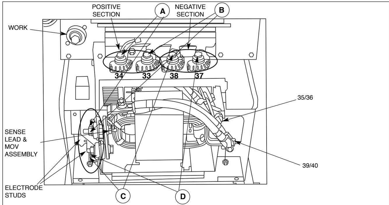
**Removal Note:** Be sure to disconnect the sense lead and MOV assembly when sliding out AC switch to access Chopper assemblies. Also, disconnect the four Amphenols behind the access door on right side of AC/DC Switch. See the *AC/DC Switch Removal Procedure*.
