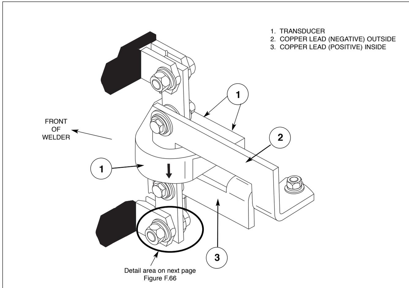
Remove both the copper bars and transducer together as a single unit. See Figure F.67.
