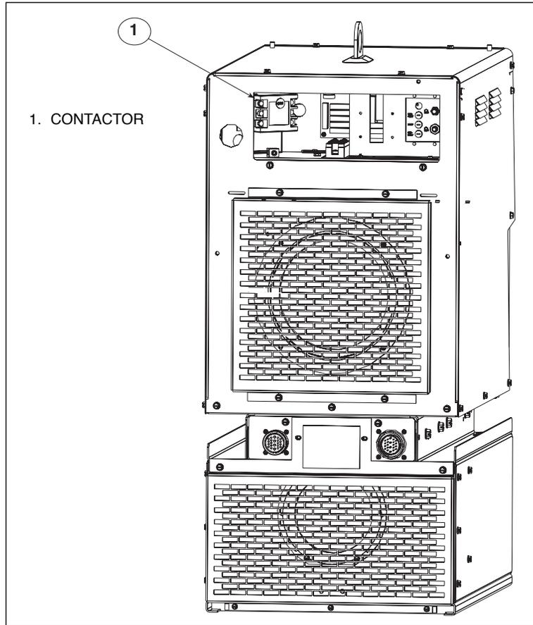
FIGURE F.38 – INPUT CONTACTOR
