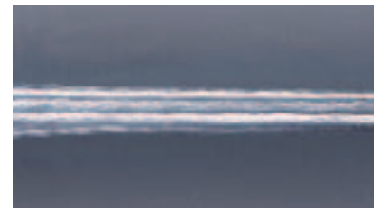
Figure 16 AC 30% Balance, 40 Hz
