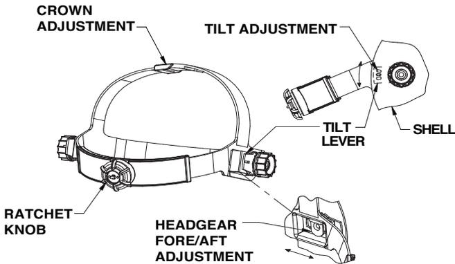
**Head Size Adjustment:** Headband tightness is adjusted by pushing in the ratchet knob and turning to adjust to desired comfort level. This knob is located at the back of the helmet. **HEAD GEAR CROWN ADJUSTMENT** is made by adjusting crown strap for vertical placement on the head and snapping the pin into the hole to lock securely in place.
