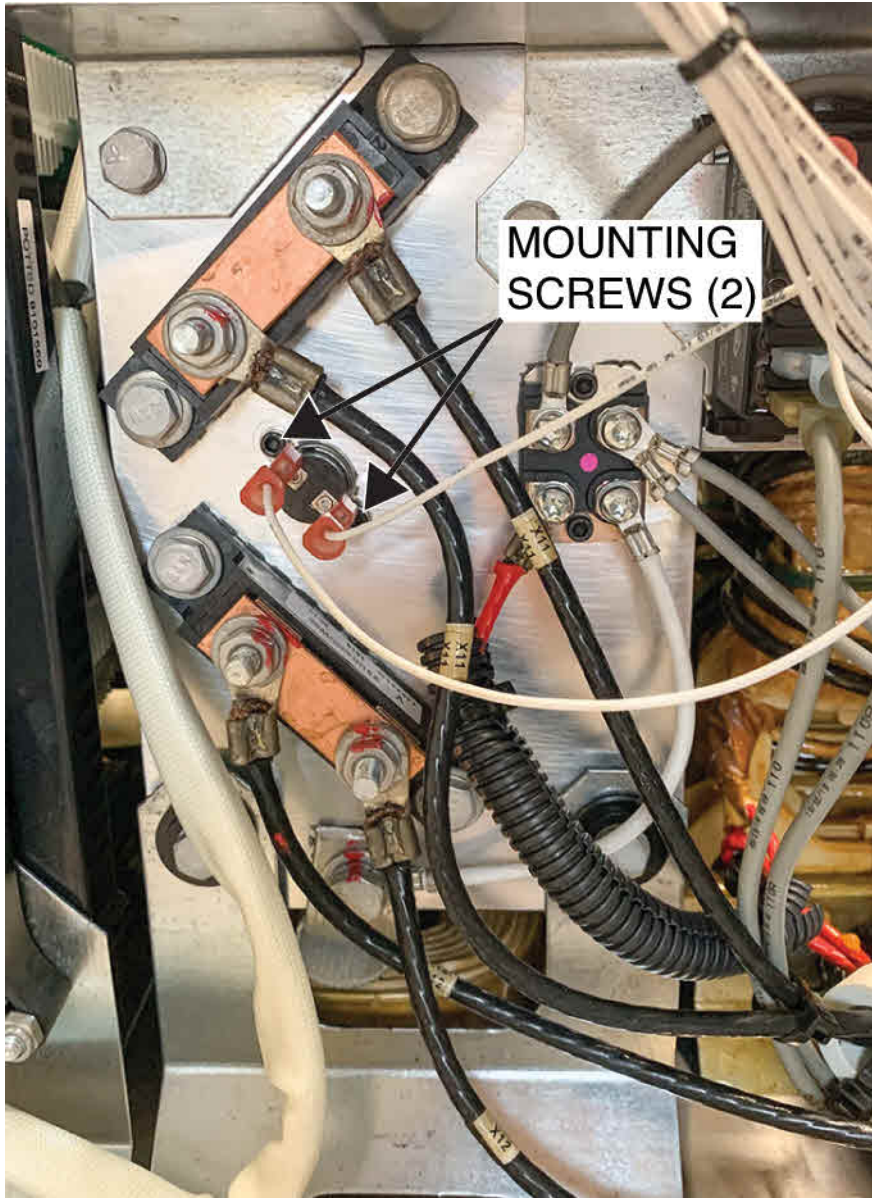
Figure 2. Thermostat #1 mounting screw locations
