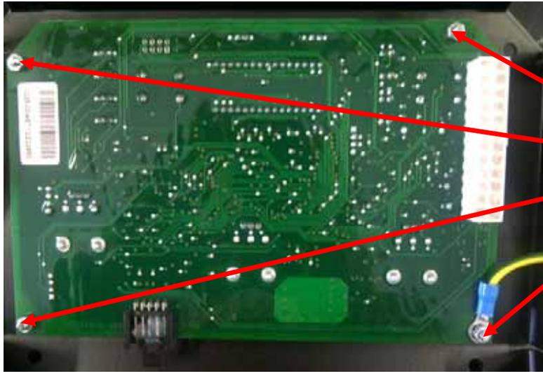
5. Using a 5,5 mm nutdriver remove the 4 nuts located on the corners of the solder side of the control board (**B**)
