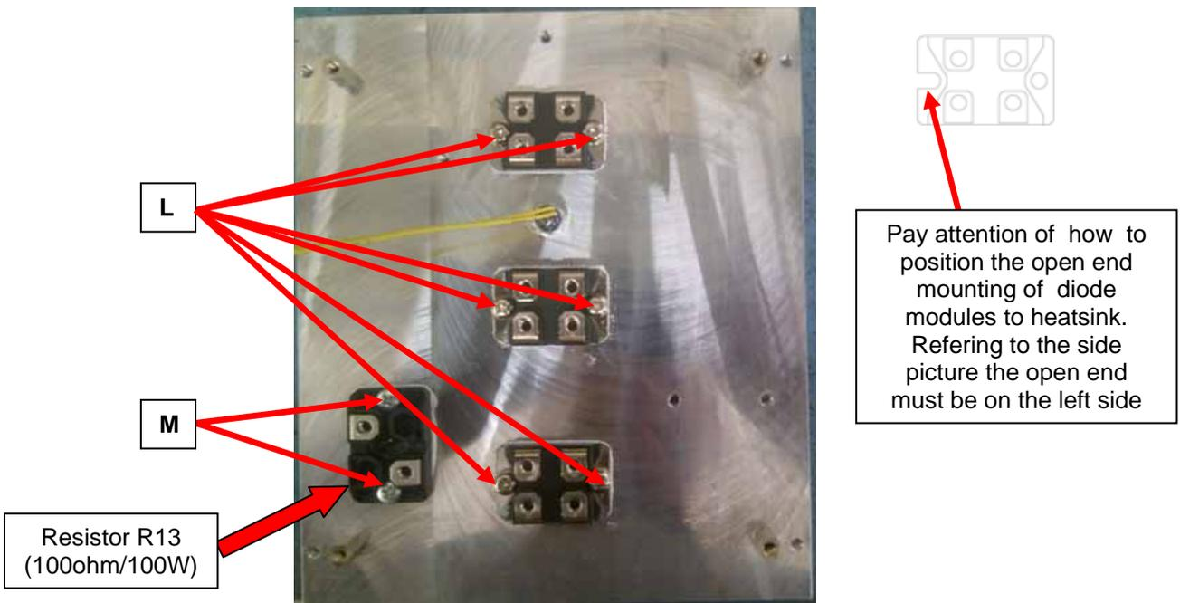
6. Remove the 6 screws (L) that fix the diode modules and the 2 screws (M) that fix the resistor R13. Keep these 6 screws in a separate place as they are different from the ones that are fixing the diode modules to the PCB. Clean the heatsink from the residual thermal compound.
