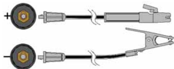
Connect the electrode cable to the (+) terminal and the work clamp to the (-) terminal. Insert the connector with the key lining up with the keyway and rotate approximately ¼ turn clockwise. Do not over tighten.
