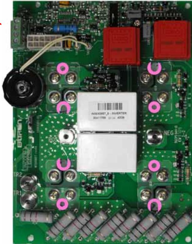
4 IGBT modules located under the inverter printed circuit
