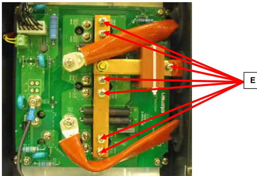
3. Unscrew the 7 screws (E) that fix the second copper bar and remove it.
