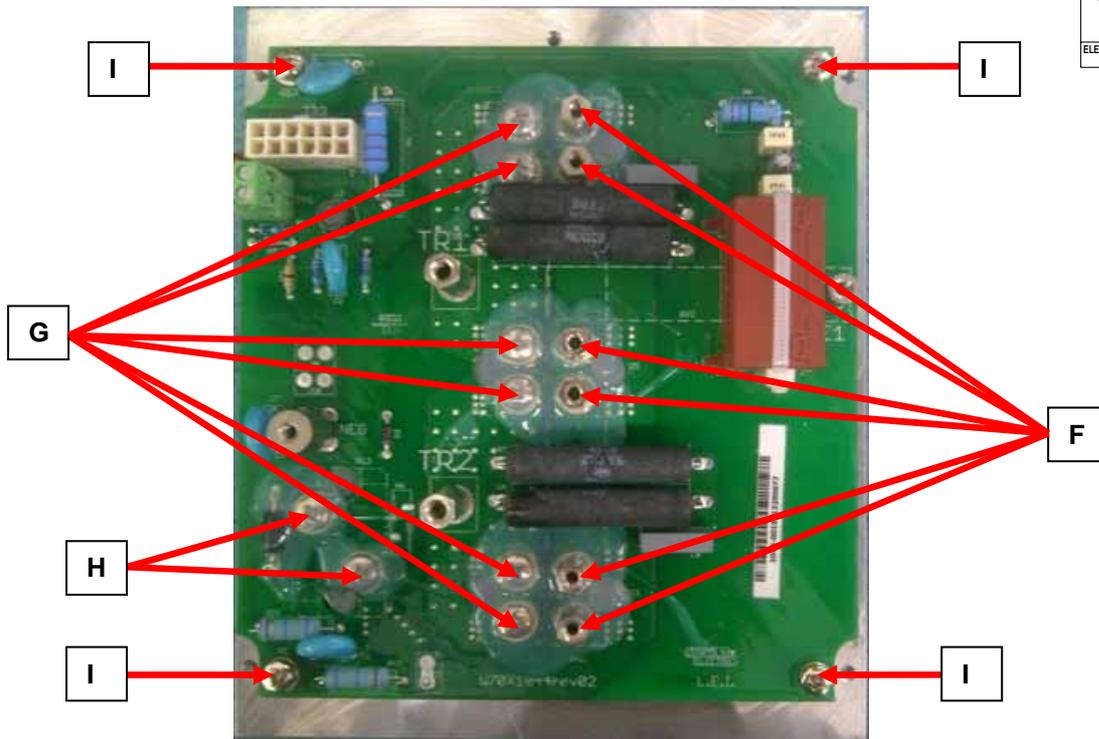
4. Remove the potting protection and unscrew the 6 spacers (F), the 6 screws (G) and the 2 screws (H).
