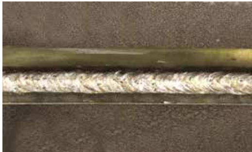
Weld bead profile [2G/PC]
