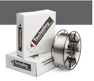
**Techalloy**<sup>®</sup> **2209** is used to weld duplex stainless steels such as (Type 2205). The welds offer excellent resistance to stress corrosion, cracking and pitting. The microstructure of the weld metal consists of austenite and ferrite. The ferrite content of the weld metal will be lower than the ferrite content of type 2205 base metal. Welding of duplex stainless steels calls for controlled welding parameters to achieve specified mechanical and corrosion resistant properties.
