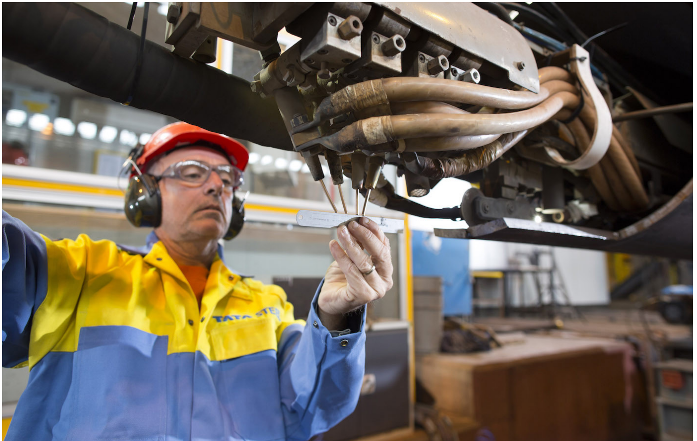
A Tata Steel operator confirms the correct lead to trail arc distance.
