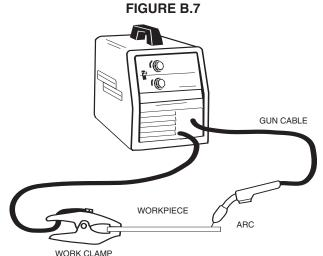
When no more welding is to be done, close valve on gas cylinder (if used), momentarily operate gun trigger to release gas pressure, and turn off the SP-175T.
