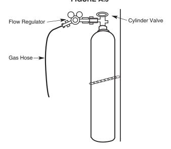
With the cylinder securely installed, remove the cylinder cap. Stand to one side away from the outlet and open the cylinder valve very slightly for an instant. This blows away any dust or dirt which may have accumulated in the valve outlet.
