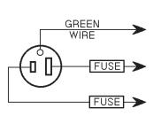
CONNECT TO A SYSTEM GROUNDING WIRE. SEE THE UNITED STATES NATIONAL ELECTRICAL CODE AND/OR LOCAL CODES FOR OTHER DETAILS AND MEANS FOR PROPER GROUNDING.
