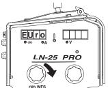
Press the set-up button to enter the WFS calibration menu.
