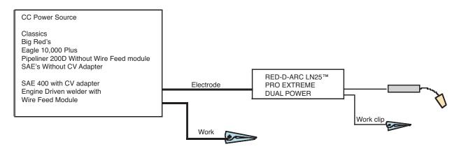
If the power source has a Remote/Local switch, place the switch in the Local position.
