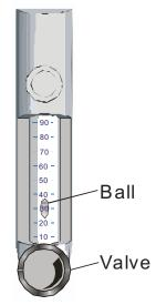
To achieve maximum flow rate, use a regulator with 30 psi or higher pressure compensation.
