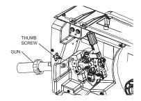
The RED-D-ARC LN25™ PRO EXTREME DUAL POWER comes with an S29807-2 gun adapter installed. (See Figure A.4a for Code 12164)
