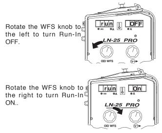
Then rotate the WFS knob to the 12 o'clock position.
