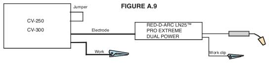
Place CV/CC switch in the feeder in the "CV" position.
