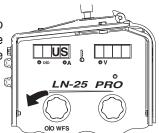
Rotate the WFS knob to the right to use "meters/minute" for the wire feed speed units.
