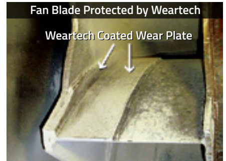
Fan blade with Weartech wear plate and coating after 12 months of service.
