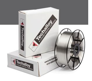
**Techalloy**® **409Nb** is a ferritic stainless steel welding wire used to weld Type 409 and 409Ti base materials. The addition of niobium improves corrosion resistance and promotes a ferritic micro-structure. For the best results, welding must be done in a low heat input procedure and is not recommended for multi-pass applications.
