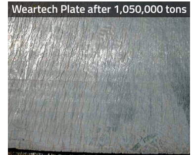
Weartech SHS9800U overlay plate has exceeded Q&T plate life by 2.9x
