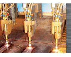
The oxy-cutting torch MACH HP is designed and manufactured in accordance with the ISO 5172 standard. It operates with several gases including: propane, natural gas and acetylene. This torch can be fitted to all Lincoln Electric machines whether equipped with a plasma installation or not. It is also available as a "retrofit" for existing machines (Lincoln Electric or other makes).
