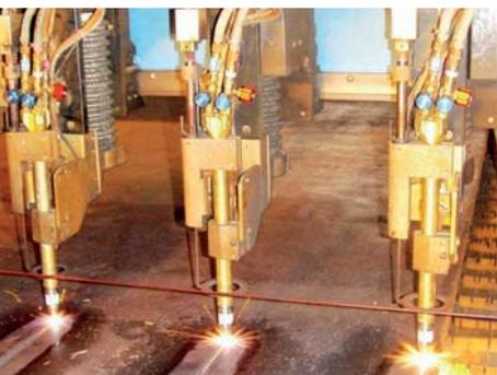
The oxy-cutting torch **MACH HP** is designed and manufactured in accordance with the ISO 5172 standard. It operates with several gases including: propane, natural gas and acetylene. This torch can be fitted to all Lincoln Electric machines whether equipped with a plasma installation or not. It is also available as a "retrofit" for existing machines (Lincoln Electric or other makes).
