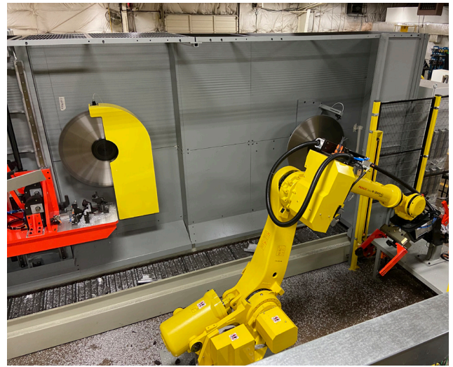
Foundry saw station with chip containment and scrap conveyor
