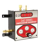
The Series 240 Manifold is designed specifically to regulate and monitor vaporized gas from cryogenic cylinders. The Series 240 Manifold prevents downtime by automatically switching over when the primary cylinder banks is depleted.
