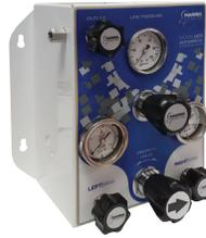
These high-purity changeover manifolds are available in brass and 316 stainless steel construction. These changeover manifolds are adjustable from 10-200 PSI. The pigtailed that are supplied with these units are leak-tight 316 stainless steel with check valve cylinder connections. The flow rate is rated at 200 SCFH of air. Alarm boxes sold separately. Comes standard with inlet/outlet isolation valve and alarm gauges
