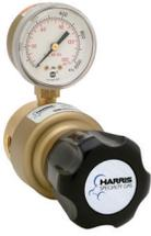
These non-corrosive general-purpose brass bar stock single stage line regulators provide a constant pressure at the point of use when the inlet pressure does not vary. The Neoprene diaphragm is perfect to provide greater sensitivity.
