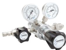
This series of two-stage, ultra high-purity regulators is designed for non-corrosive analytical and process applications requiring precise, stable delivery pressure control. The two-stage design yields a delivery pressure of less than 0.05/100 psi inlet change.
