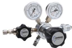
These chrome plate brass, single-stage, ultra high-purity regulators are recommended for non-corrosive analytical and process applications where precise flow control is not critical. A specially designed, convoluted, stainless steel diaphragm provides good regulating
