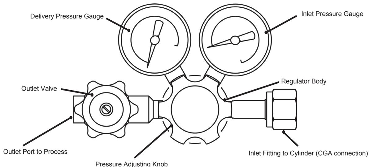
two-stage regulator reduces the pressure in two steps, either may be suitable for the application based on the desired pressure control. Single-Stage regulators are best suited for applications where manual periodic adjustment of the delivery pressure settings is not a problem and the inlet pressure remains constant, such as the case in gas withdrawal from liquid cylinders.
