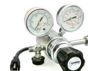
This regulator can be used with gases that encounter the Joule-Thompson effect created in pressure drops across the internal orifices in a regulator. The regulator will maintain the gas in the vapor phase by supplying heat at the regulator's internal orifice while providing a constant delivery pressure.
