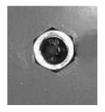
This switch must not in any case be used as an activation button. It must only be used in emergencies.
