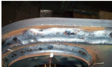
Example of bad wire placement
