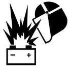
• **CONNECTING A BATTERY CHARGER** - Remove battery from welder by disconnecting negative cable first, then positive cable and battery clamp. When reinstalling, connect negative cable last. Keep well ventilated.
