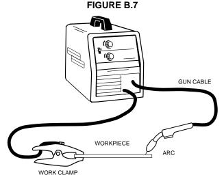
When no more welding is to be done, close valve on gas cylinder (if used), momentarily operate gun trigger to release gas pressure, and turn off the SP-170T.
