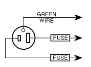
CONNECT TO A SYSTEM GROUNDING WIRE. SEE THE UNITED STATES NATIONAL ELECTRICAL CODE AND/OR LOCAL CODES FOR OTHER DETAILS AND MEANS FOR PROPER GROUNDING.
