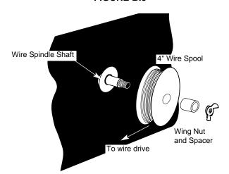
**Note:** The brake should be adjusted with a spool of wire installed. When properly adjusted it should move freely but not coast.
