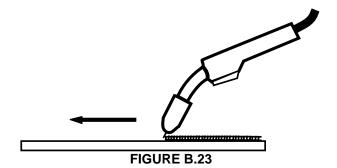
When using the GMAW process on light gauge material, weld from right to left (if you are right handed). This results in a colder weld and has less tendency for burn through.
