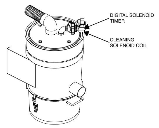
Figure F.17 - Cleaning solenoid and digital timer location
