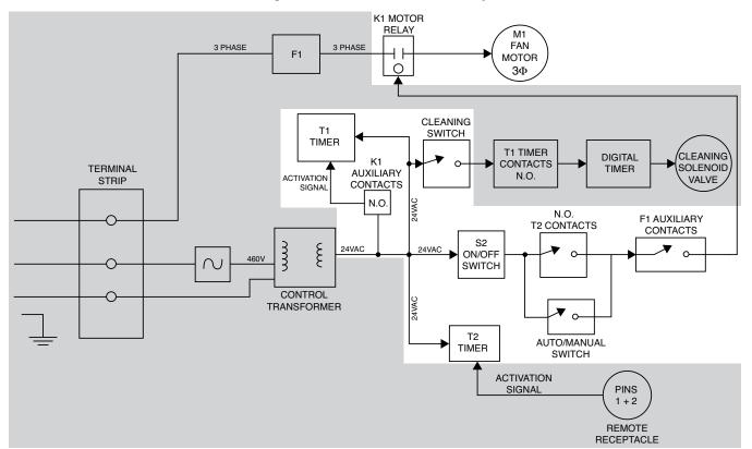
Figure E.3 - Motor control circuitry
