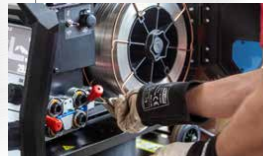
Full access for wire spool installation
