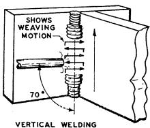
If vertical down welding is employed the arc is struck at the top with the electrode slanting below the horizontal about 20 degrees. The speed of travel should be fast enough to prevent the metal and slag from becoming too fluid, as it will then tend to flow out of the craters and cause interference with the arc. For best results a short arc should be used.
