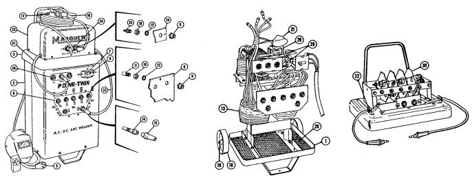
The following parts list and the above illustrations completely identify all parts of the Marquette Model 12-100 Welder. Use this list when ordering replacement parts.
