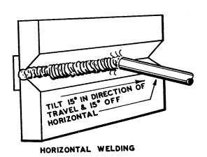
Horizontal butt joints on sheet metal up to 1/16'' thick can be made from one side. If the seam has numerous gaps, use a back-up strip. Allow a slight gap between sheet metal around  $\frac{1}{8}''$  thick and weld from both sides. All metal 3/16'' thick and over should be beveled and welded with a number of passes.
