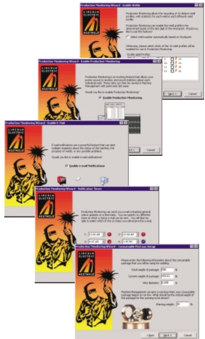
The Production Monitoring Wizard guides the user through setting up limits and e-mail configuration
