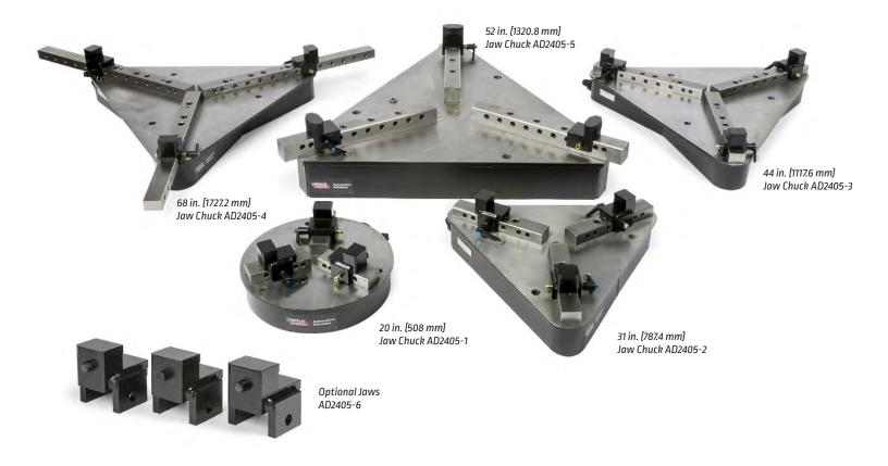
Lincoln Electric® jaw chucks for welding positioners are designed and built to include single point cam operation and adjustable quick change reversible jaws that can be positioned for small and large diameter workpieces. A completely enclosed face prevents flux and weld spatter from impairing the operation of the gripper.
