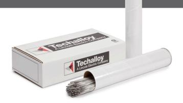
**Tech-Rod**® **2209** is used to weld duplex stainless steels such as (Type 2205). The welds offer excellent resistance to stress corrosion, cracking and pitting. The microstructure of the weld metal consists of austenite and ferrite. The ferrite content of the weld metal will be lower than the ferrite content of type 2205 base metal. Welding of duplex stainless steels calls for controlled welding parameters to achieve specified mechanical and corrosion resistant properties.
