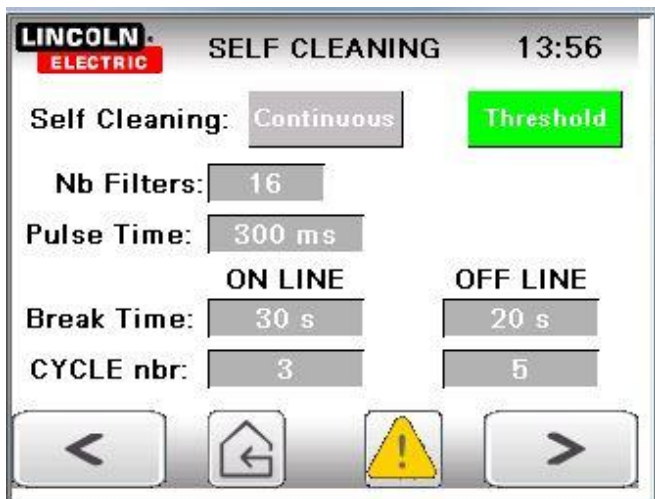
Unclogging setting screen
