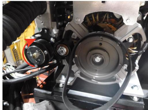
**Step 20:** When installing the replacement belt, make sure the grooves of the belt line up and go underneath the small wheel.
