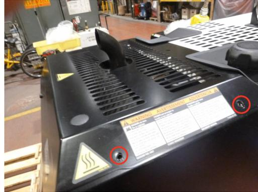
**Step 5:** Slide the RANGER AIR 260MPX/330MPX left door panel towards the rear of the machine and remove.
