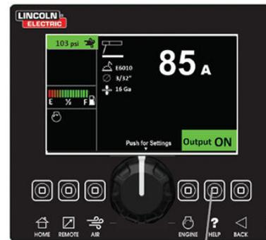
Rotate the knob to choose the electrode type. Press the knob to select. To turn off Ready.Set.Weld, select “Manual Entry”.
