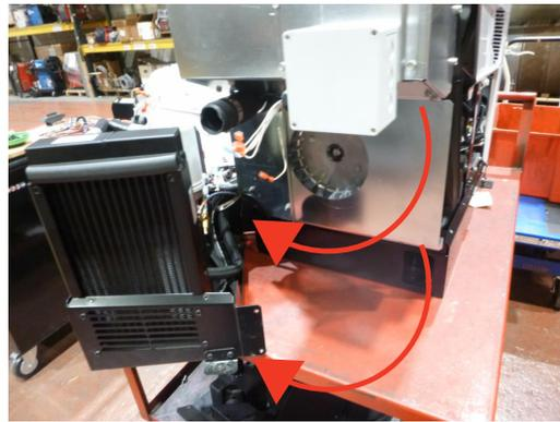
**Step 15:** Remove the 2 screws that secure the bottom of the back plate to the machine..
