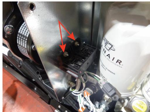
**Step 13:** Locate and remove the nut on the grounding stud then remove the ground lead from the stud. Cut the zip tie holding the harness together to separate the ground lead from the harness.
