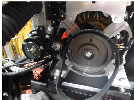
**Step 21:** Rotate the clutch counterclockwise back into position and place a 3/8 in socket into the square hole to hold it in place.
