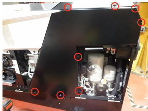
**Step 4:** Locate and remove the 4 screws that secure the roof grill to the machine.
