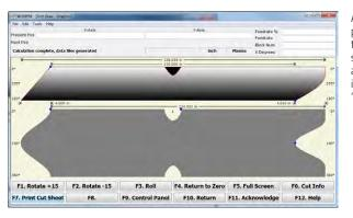
After calculating the cut paths and checking for errors, the optional WinMPM design software provides a rolling animated view of the pipe as it will be cut as well as an "unrolled" cutting pattern.
