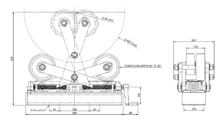
x-rotator 1t - diameter: 60-1020mm
