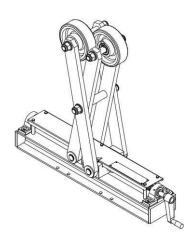
These X-rotators can be mounted on idler lorry (W000274920) in order to facilitate the transversal movement.
