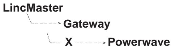
Communication lost; a chart is displayed with the status of communication between **LINC-MASTER (PC104) <-> Gateway <-> POWERWAVE**.
