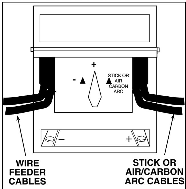
The MULTI-PROCESS SWITCH has two sets of output terminals. You connect the wire feeder unit cables to the set of terminals on the left side of the box and the stick or air/carbon arc cables to the set of terminals on the right side (facing the front of the machine) as shown in Figure C.1. The output terminals are protected against accidental contact by hinged covers.
