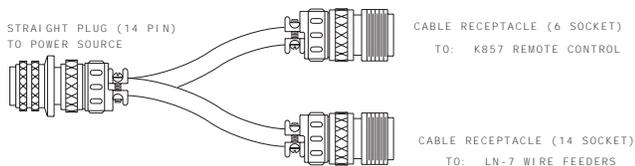
A "V" cable 12" (.30 m) long to connect a K857 Remote Control (6-pin connector) with an LN-7 wire-feeder (14-pin connector) and the machine (14-pin connector). If a remote control is used alone the wire-feeder connection is then not used.
